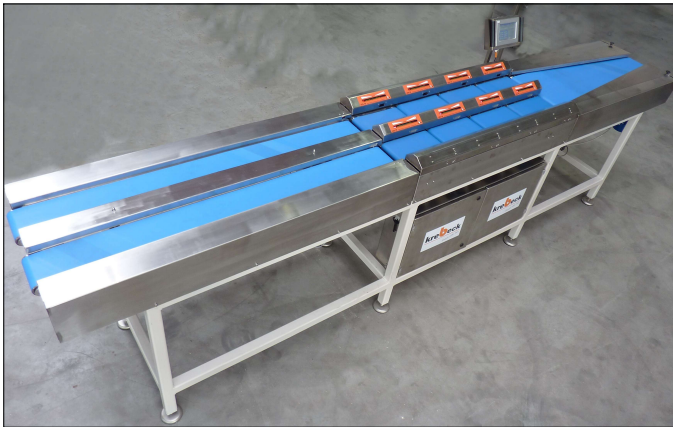
Weighing line with 8 weighing units
