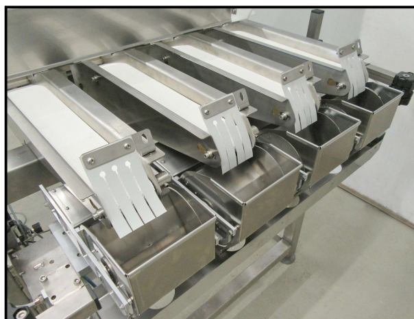
Dosing arms with weighing chamber and butterfly valve
