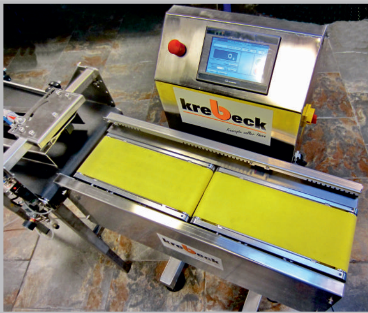
Check weigher KR400 with touch screen and belt units for inbound control and weighing.
