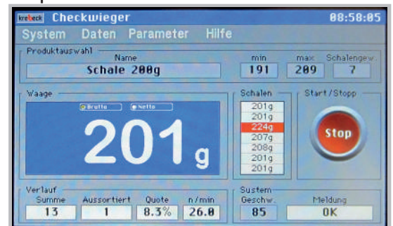
Touch screen of the operator unit with display of actual and last seven weighing results plus other product details.
