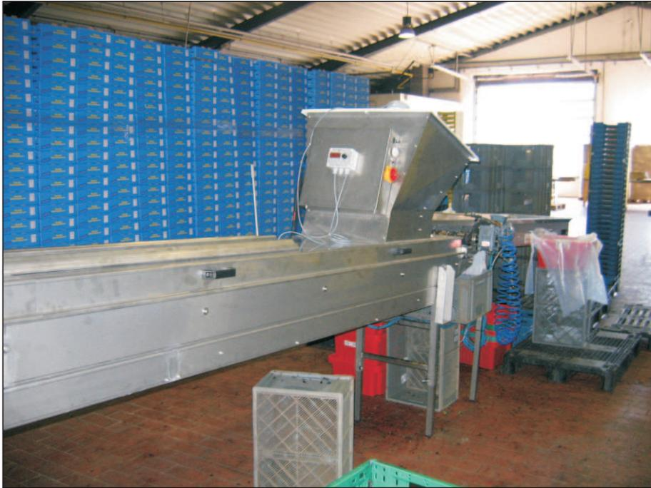
Drying Belt with hot-air unit and Conveyor Belt.
