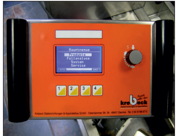
Input Device for Dosing Process Control. Products from 0,100 - 8,00 kg can be handled
